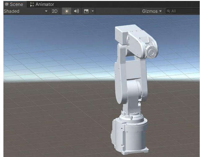
Fig. 1 Modeling of the Mitsubishi RV-2SDB Robot
